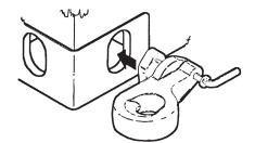
Insert lug into bottom-side I.S.O. corner casting hole.
